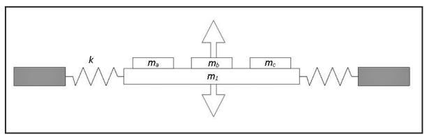
Figure I: The diaphragm schematics show Total mass =  $m_1 + m_a + ... + m_i$
