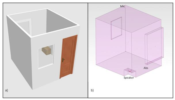
Figure II: A small room with easily determined room modes was used for testing (a). A speaker was placed in one corner and a microphone was placed in the opposite corner (b).
