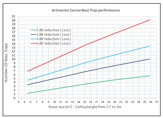
Figure XVII: We can conclude a direct ratio between the number of absorber units, volume, and the decibel reduction in each room.
