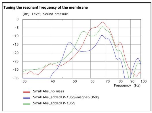
Figure V: Measurements of mobility with the Laser Doppler Velocimeter (LDV) show the tuning of the absorber.
