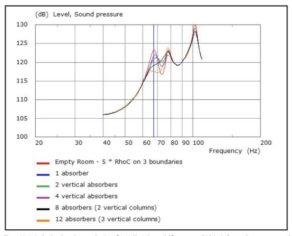
Figure XI: A single absorber gives a reduction of 1.66 dB at the modal frequency, which is similar to what was measured.
