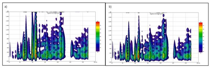
Figure IX: The reverberation time (RT) for an empty room (a) and the RT with three bass trap units (b). We can see a significant difference at 60 Hz—the RT drops from over 2.4 seconds to just under 1 second. There is significant reduction up to 140 Hz. The overall peak energy level also decreases over the frequency range.
