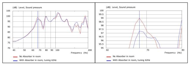
Figure IV: These are the performance results for the single unit in the room..
